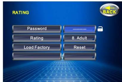
**Password:** first set the rating (in RATING setting). Then select the Password setting, press the numeric buttons on the remote control to set the 4-digit password to protect the parental lock from being changed.
