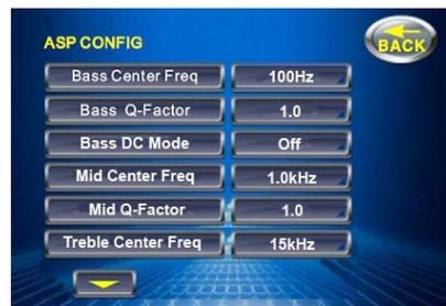
**Bass center frequency:** select the Bass center frequency according to the audio source disc: 40 Hz, 50 Hz, 60 Hz, 70 Hz, 80 Hz, 90 Hz, 100 Hz, 120 Hz, 150 Hz.
