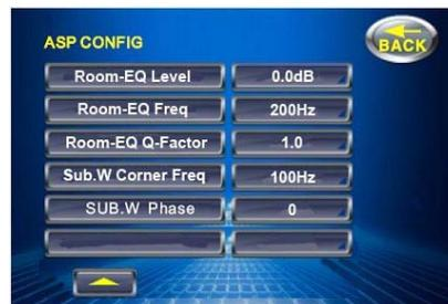
**Room-EQ Level:** adjust the gain of Room EQ (0.0dB, 1.0dB, 2.0dB, 3.0dB, 4.0dB, 5.0dB, 7.0dB, 9.0dB).
