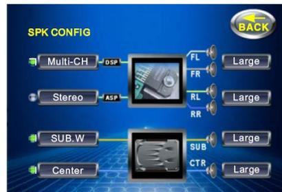
**Multi-Ch:** set up the front speakers: Large (suitable for speakers with good bass output), Small (for speakers with bad bass output).
